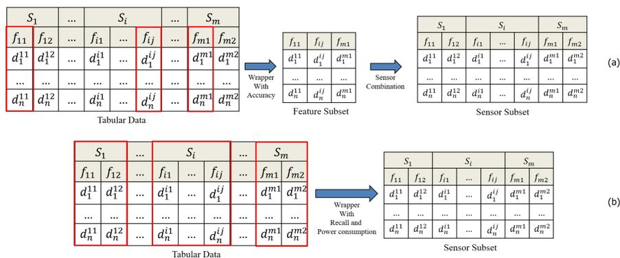
Figure 1: Comparison of sensor selection method between (a) conventional method and (b) proposed method
