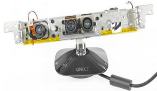
Figure 4: Kinect Without its Plastic Housing, Showing from Left to Right the Infrared (IR) Emitter, the RGB Camera and the IR Camera [15].
