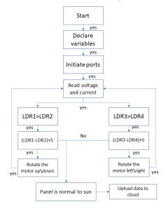
Figure 5: Flow Chart of Solar Tracker System
