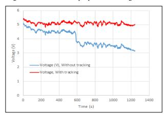
Figure 6: Voltage Comparison of the Dual with Fixed Angle Design
