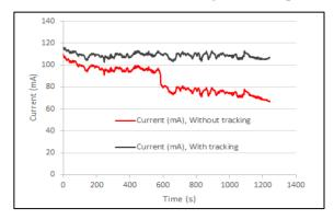
Figure 7: Current Performance of the Dual Axis Solar Panel Tracker in Comparison with the Single Axis Circuit
