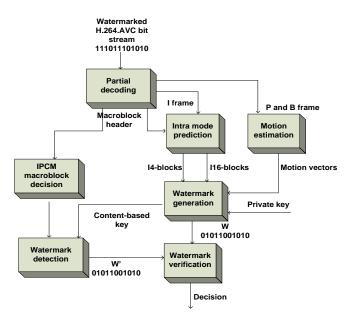
Figure 4: Block Diagram of Watermark Detection and Verification Process
